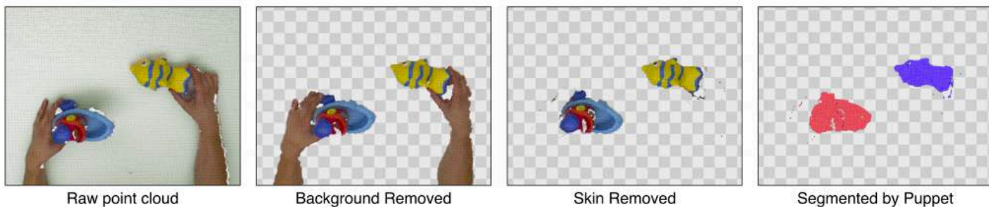
Figure 6. Steps of point-cloud segmentation. Beginning with the raw point cloud from the Kinect, our segmenter removes the background and the puppeteer's skin, and finally produces separate point clouds associated with each puppet.
