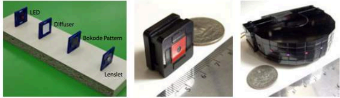
Figure 4: Photos of Bokode prototypes discussed in the paper: (left) exploded view of our active illumination prototype, (center) an assembled Bokode, and (right) our compound superposition eye (Antarctic Krill) prototype for an ultra wide angular range.
