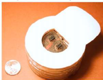
Figure 3: A Sensetable puck, with a socket for attaching a dial or modifier. A US quarter is shown for scale.
