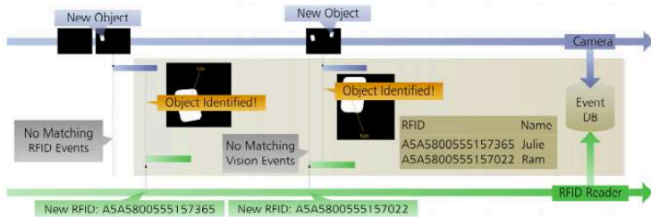
Figure 6: The fusion pipeline. As new events appear, the system tries to match them with previously unmatched events in order to associate localize and identify shapes on the surface.
