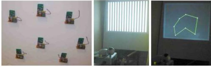
Figure 4: (a) A tagged surface, (b) One frame during Gray-code projection, (c) Correctly-placed projected augmentation.
