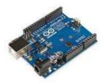
a single-board microcontroller, intended to make the application of interactive objects or environments more accessible
