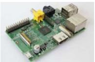
The Raspberry Pi is a credit-card-sized single-board computer developed in the UK by the Raspberry Pi Foundation with the intention of promoting the teaching of basic computer science in schools
